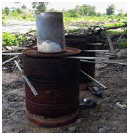
Photo 1. Burning rice husk to make biochar
